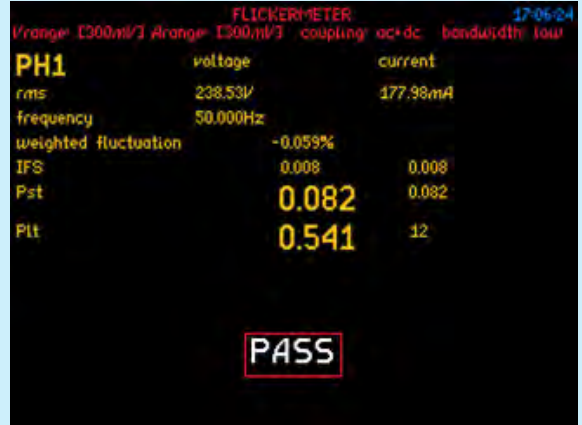
After the test is complete, the unit will display a Pass or Fail message. A screen shot can be downloaded to software, alternatively the test can be controlled and monitored in software.
